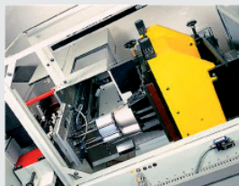
Die-cutting with counterpressure
